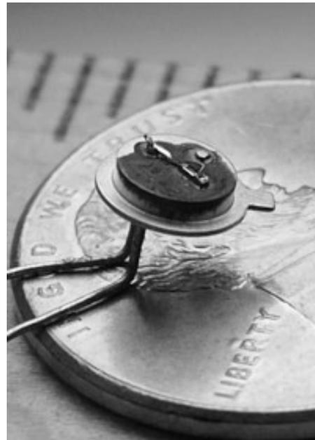
The red light-emitting diode (LED) developed by Nick Holonyak Jr. in October 1962 uses a crystal of gallium arsenide phosphide alloy—the small rectangular block on the top of the gold-plated platform.
