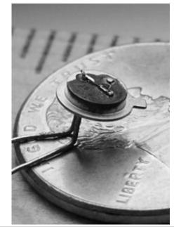
The red light-emitting diode (LED) developed by Nick Holonyak Jr. in October 1962 uses a crystal of gallium arsenide phosphide alloy-the small rectangular block on the top of the goldplated platform.
